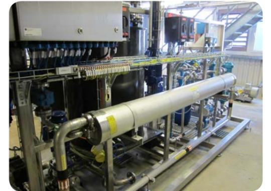
For example **CLARIANT, Gersthofen/DE** – Separation and recovery of nitrous additives from the production of polymer additives.
