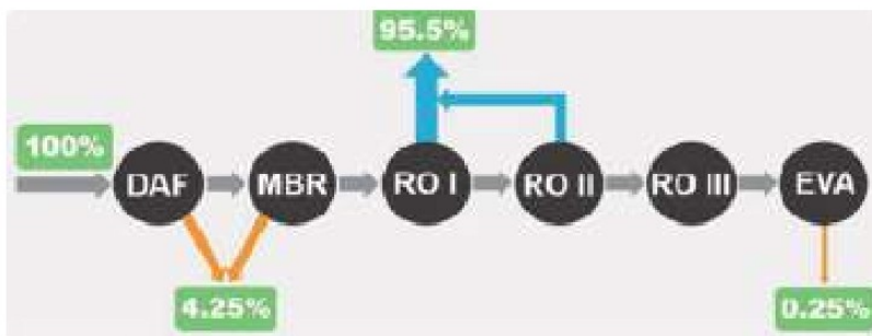
Figure 5: Process chain of the ZLD plant as well as the percentage of final products leaving the process.
