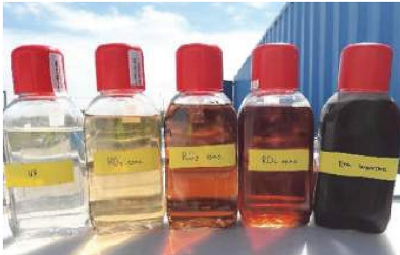
Figure 4: Concentrates from the respective process stages, from UF permeate (left) to evaporator concentrate (right).
