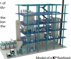
bed plant for decentralized thermal utilization of waste for 1 MW<sub>th</sub> or more
