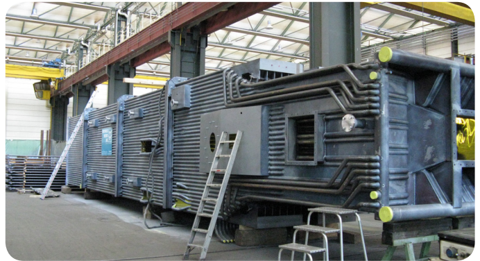
Manufacturing of the boiler at WEHRLE
