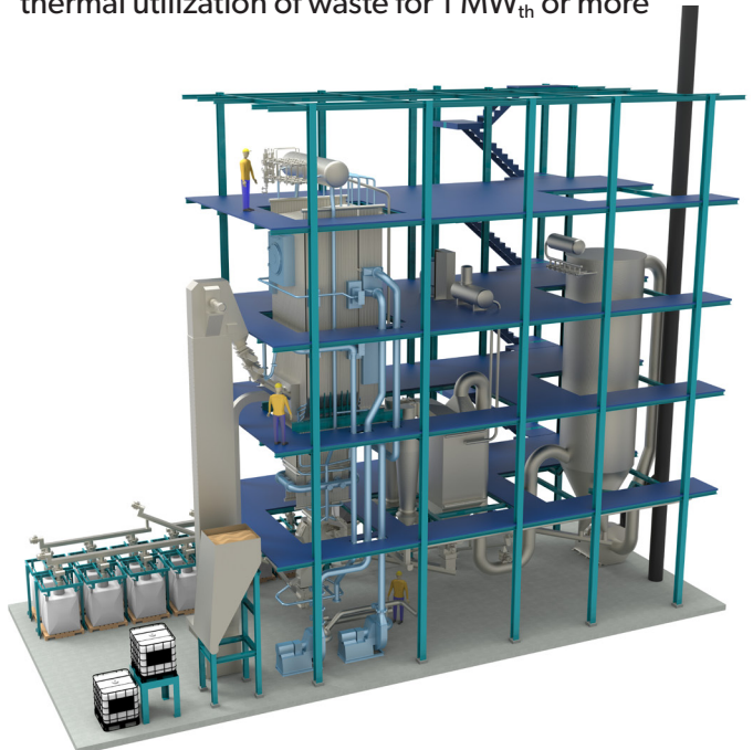
Model of a K 3 fluidized bed plant for decentralized thermal utilization of waste for 1 MW th or more
