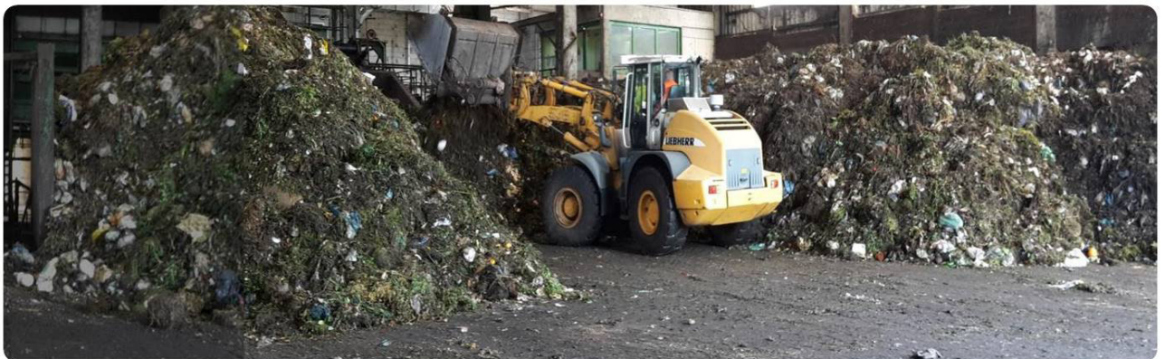
Example of decentralized thermal utilization: Disposal of screen overflows from a biogas plant
