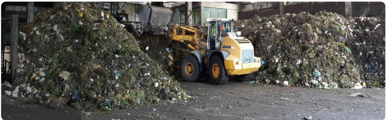
Example of decentralized thermal utilization: Disposal of screen overflows from a biogas plant
