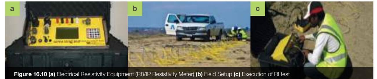
Figure 16.10 (a) Electrical Resistivity Equipment (R8/IP Resistivity Meter) (b) Field Setup (c) Execution of RI test
