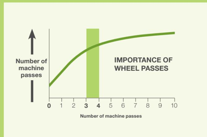
Figure 8.6 Compaction and Number of Passes
