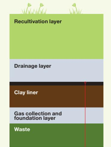
Figure 19.3 Examples of a simple soil cover and a state-of-the-art barrier layer
