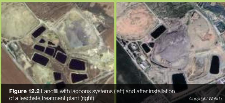
Figure 12.2 Landfill with lagoons systems (left) and after installation of a leachate treatment plant (right)
