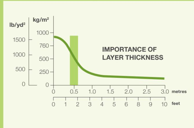
Figure 8.5 Optimum Compaction and Waste Layer Thickness
