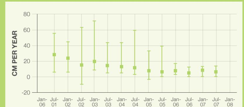
Figure 19.2 Settlement (average and range of 17 measurements points) on a 22 ha landfill since operation ended in 2000
