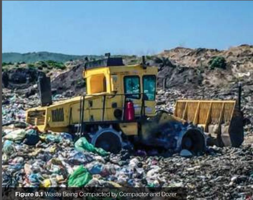
Figure 8.1 Waste Being Compacted by Compactor and Dozer
