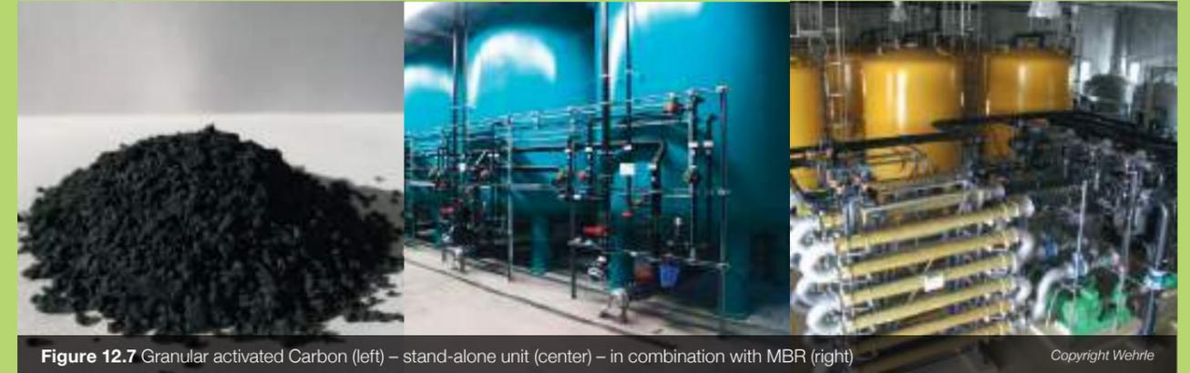
Figure 12.7 Granular activated Carbon (left) – stand-alone unit (center) – in combination with MBR (right)
