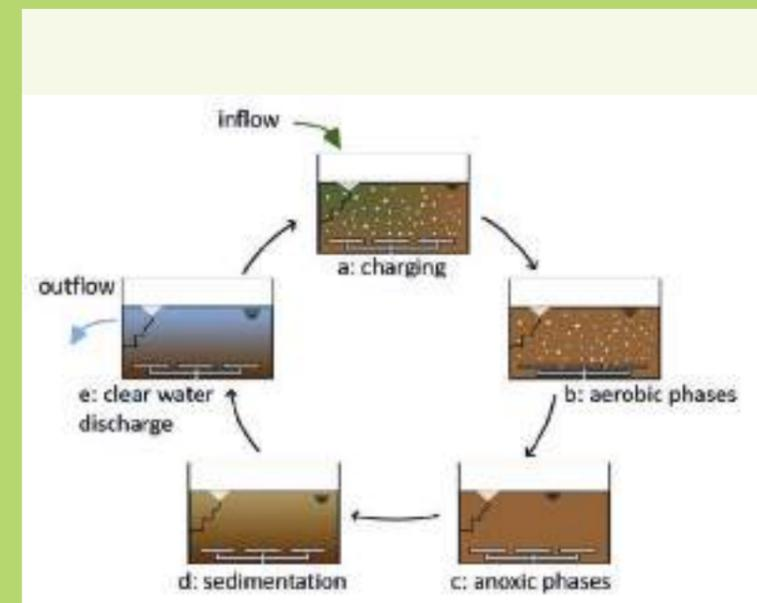
Figure 12.8 Biological “elimination” technologies: SBR process
