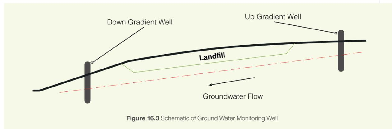
Figure 16.3 Schematic of Ground Water Monitoring Well
