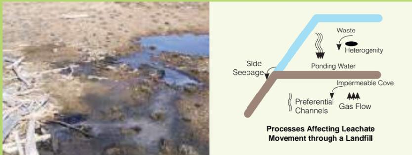
Figure 16.7 Leachate seepage through side slopes (Alam, 2016)
