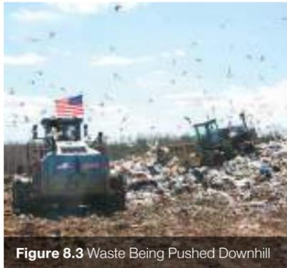
Figure 8.3 Waste Being Pushed Downhill
