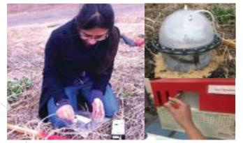
Figure 16.1 Flux Chamber Sampling and Determination of Concentration with Gas Chromotograph (Samir, S., 2014)
