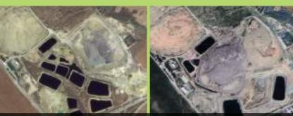
Figure 12.2 Landfill with lagoons systems (left) and after installation of a leachate treatment plant (right) Copyright Wehrle As leachate forms and passes through the waste, organic and inorganic compounds become dissolved and suspended in the leachate. This process can be likened to the process of passing water through coffee grounds to make coffee.
