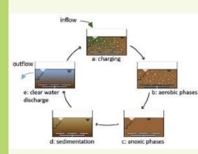
Figure 12.8 Biological "elimination" technologies: SBR process
