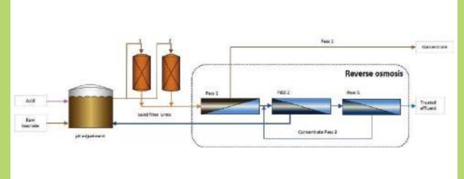
Figure 12.5 Reverse Osmosis (RO) technology: flow chart of a 2-pass unit
