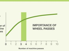
Figure 8.6 Compaction and Number of Passes
