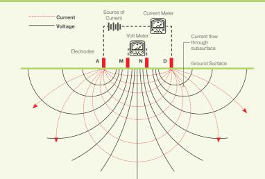
Figure 16.9 Equipotential and Current Lines for a Pair of Current Electrodes A and B
