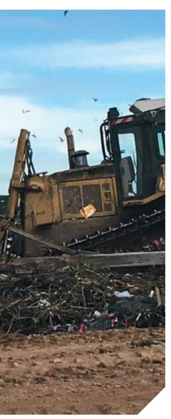
Bulky waste that is able to be crushed or shredded (e.g. old furniture) should be deposited at the bottom of the working face, so as to be cut and crushed by the bulldozer (Figure 7.4).
