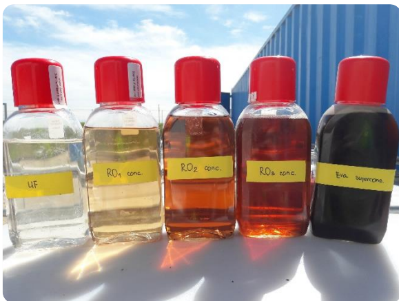
4) Concentrates from the respective process stages, from UF permeate (left) to evaporator concentrate (right).
